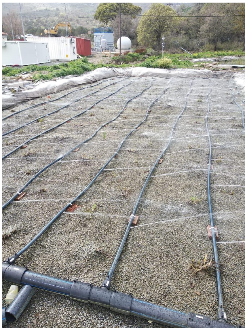
Figure 4.25. Testing CWs feeding system
